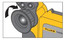
Figure 1-5. Focusing the Camera
