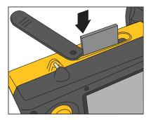
Figure 1-4. Inserting a Memory Card
