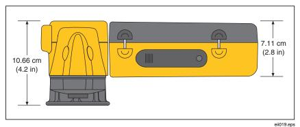
Figure D-1. Camera Dimensions
