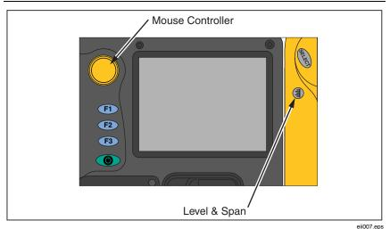
Figure 1-7. Setting the IR-Fusion® Blend Level
