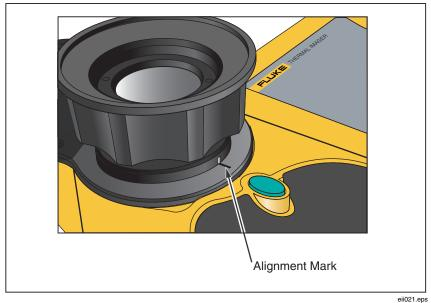
Figure 5-1. Aligning the 20-mm Lens
