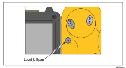
Figure 1-6. Setting the Level and Span
